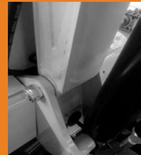
Pivot at base of boom cylinder
